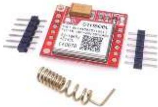
Gambar 4 Modul GSM SIM800L [12]
