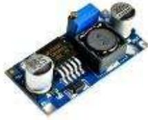
Gambar 5 Step-Down Voltage Regulator [17]
